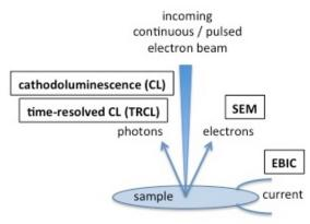
measurements (TRCL) that provide valuable information on carrier dynamics and lifetime. Our CL/TRCL setup has state-of-the-art specifications and is extremely versatile: wide ranges of wavelengths (200nm-1600nm) and temperatures (10K-350K), time-resolved measurements (temporal resolution 10ps). In addition, its very high collection efficiency on a wide field of view is perfectly adapted to CL and TRCL mapping of a wide variety of photovoltaic (PV) materials.
